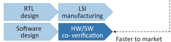
Fig. 1 Hardware and software development. System verification (HW/SW co-verification) during LSI manufacturing using RTL (register transfer level) design data enables faster time-to-market for system products.
